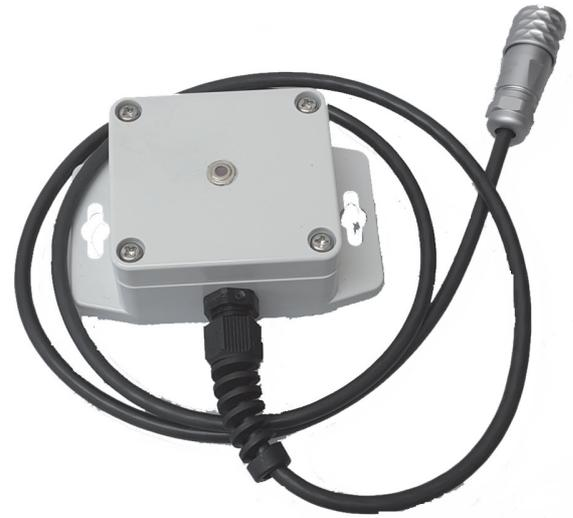
The TruSense Input modules are an I2C based module with memory and the interface to the sensors. When an Input module is connected to a TruSense logger the logger reads the Input Module's memory and this gives the logger all the information on the sensors that may be attached to the module.
